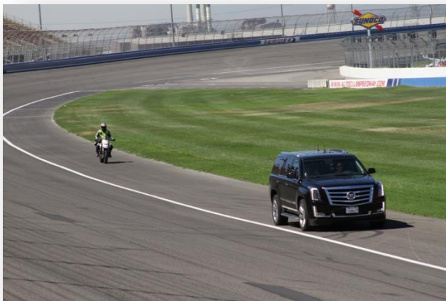
FIGURE 4: BLIND SPOT MONITORING TEST WITH MOTORCYCLE TARGET VEHICLE. THIS SCENARIO IS ILLUSTRATING THE PASS-FROM-BEHIND TEST
